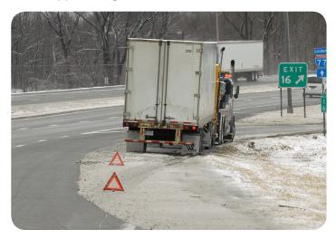
**Within 500 feet of a hill, curve, or obstruction.** A device should be placed:
